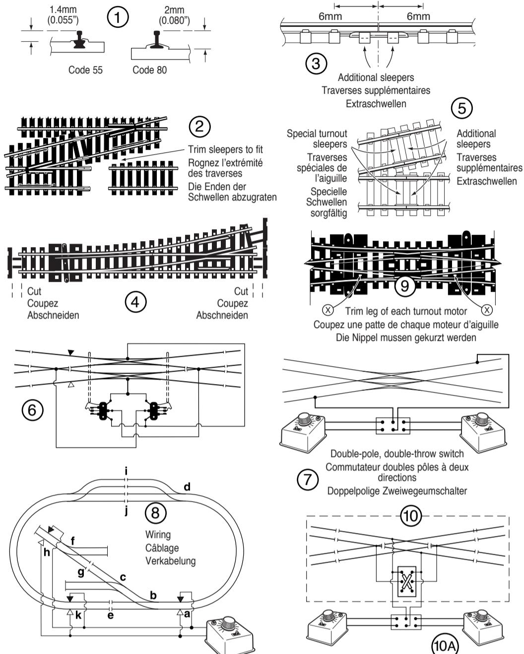
Turnouts are ready for immediate use – separate levers are not necessary. For remote control, the Peco Lectrics Turnout Motor (PL-10) simply clips underneath and is operated by a special Switch (PL-26) or the Probe (PL-17) and Stud (PL-18) system.
